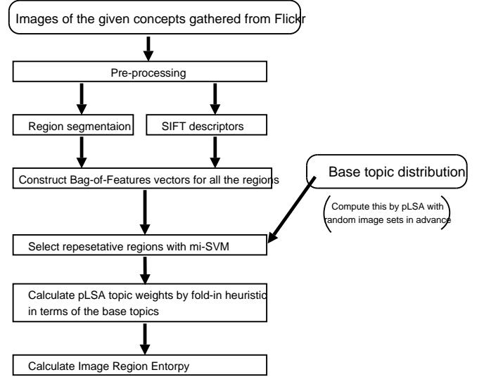
**Figure 1: Flow diagram of the procedure to obtain the “image region entropy”.**
