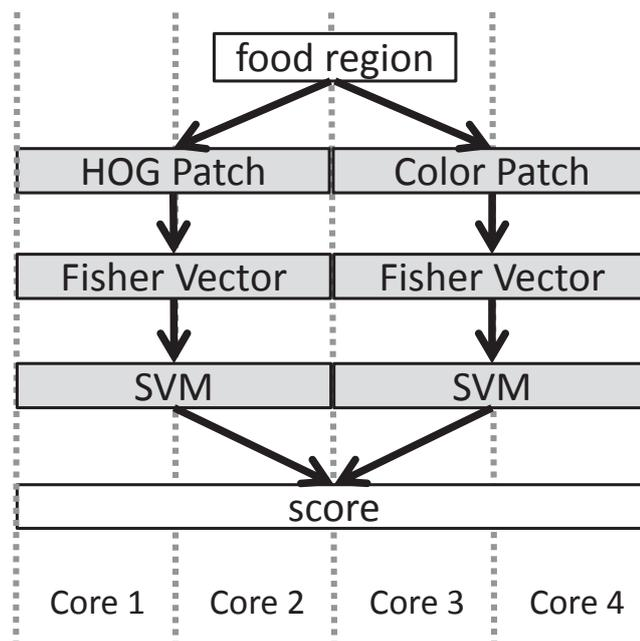
**Fig. 5** Processing flow and assignment on CPU cores for the system using a HOG patch and a Color patch with Fisher Vector
