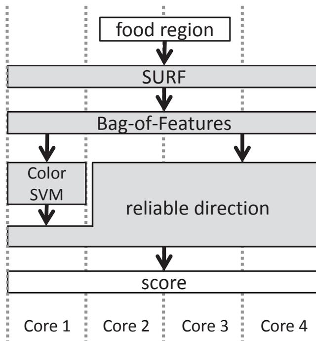
**Fig. 4** Processing flow and assignment on CPU cores for the system using bag-of-features and color histogram.
