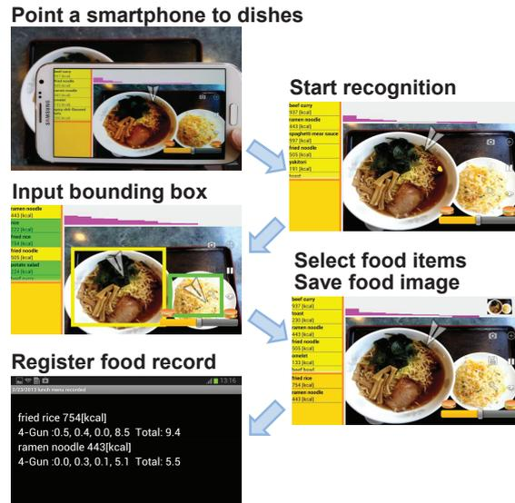
Fig. 2 System process flow
