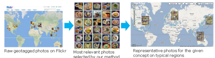
Figure 1: After collecting geotagged photo related to the given concept by the text-tag-based search, we remove noise images, cluster regions and select regional representative images.
