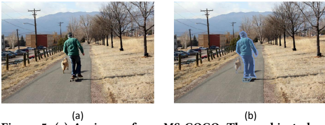
Figure 5: (a) An image from MS-COCO. Three object class labels, “person”, “dog”, and “skateboard”, are attached to this image. (b) Pixel-level ground-truth for those three classes.
